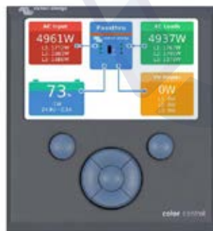
Color Control GX, showing a PV application
